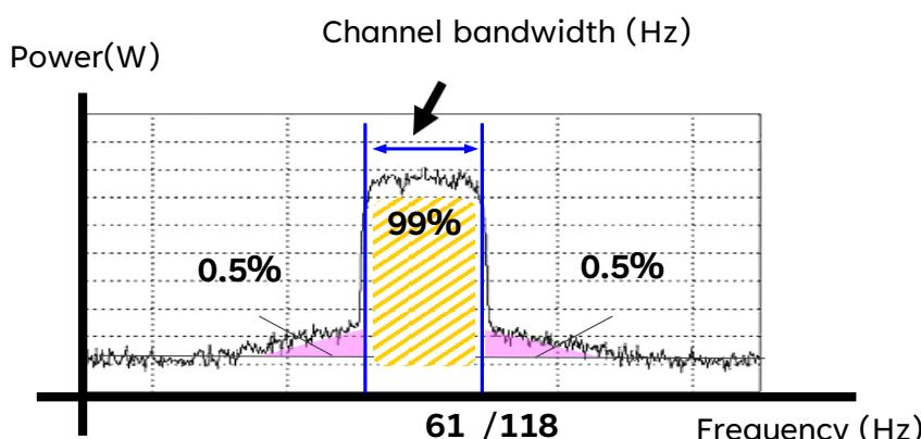
Figure 1 Spectrum analyser waveform
